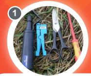
Sheath Stripper P/C 9728 Microduct Rotational Cutter P/C 7299 Heavy Duty Scissors P/C 7039 Flat Head Screwdriver
