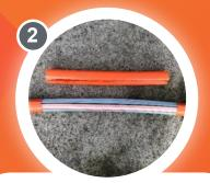
Remove the sheath but do not throw away. The selection of microduct can now be made.
