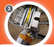
Feed the fibre until LFBT is completely through seals and clamp and attach fibre seal. Close drive wheels to secure.
