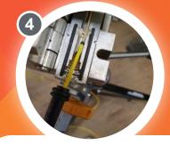
Attach microduct to GS150 and secure, closing the fibre guides and tightening screw. Perform a crash test before installation.
