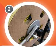
Attach fibre reel to stand, tighten the screw to secure the reel. Adjust depth of resistance screw to control speed of unwinding.
