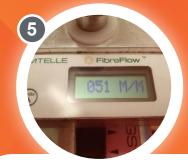
Blow QWKlink into the route at a maximum speed of 50 m/min.
