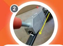
Pull the tool towards your body, when the back of the tool reaches the second mark start to lift the back of the tool.
