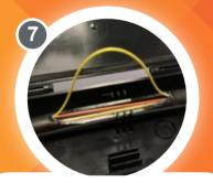
The fibres can now be selected to be pushed or pulled back to the desired drop microduct.
