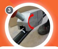
When lifting the tool, do not pull straight up, lift the handle forward as the tool is pulled back this will give a tidy window cut.
