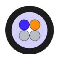
2F Fibre with 2 Mechanicals 1.047 g/m 1.05 mm ITU-T G657 A2
