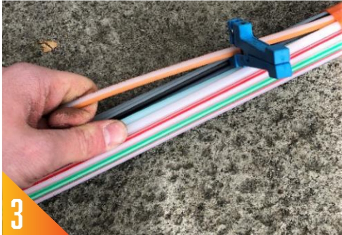
3 Once the blade is set, position the cutter where the cut is needed. Rotate 2-3 times, enough to score the microduct.
