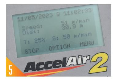
Perform the normal cable blowing checks and procedures for installation. Do not exceed 50m/min installations speed @ 15bar pressure.
