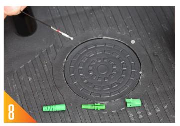
Use the QWKlink accessories from Step 1 and following the enclosed instructions to assemble the optical connectors at both ends.
