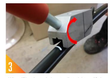
When lifting the tool, do not pull straight up, lift the handle forward as the tool is pulled back this will give a tidy window cut.
