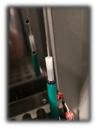
Push the activation collar down to secure the ELF. The ELF is now activated, and fibre secured.
