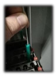
Gently pull outwards approx. 20mm of free moving fibre unit.
