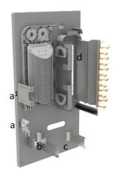
The Cabinet is supplied with a main feeder cable retention bracket (a) that can accommodate up to 3  $\times$  23mm cables. This is ideal for loop through application and located right below the loop tube storage bracket(a<sup>1</sup>). The cable can be secured additionally via the strength member or by fixing the aramid yarns to the anchoring point.
