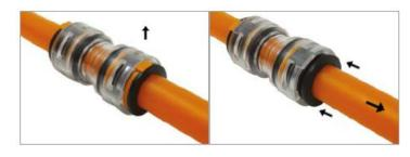
In order to disconnect the microduct from the connector, remove locking clip first, then push the collet towards the connector body and pull the microduct keeping the collet pushed against the connector body.
