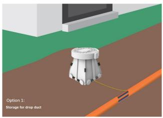
Bemarcation point between 2 or 4 homes as slack storage for drop ducts or drop cables.
